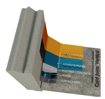
Floor / wall corners (cold joints) are a weaker area of any concrete structure, so they are more likely to leak.
