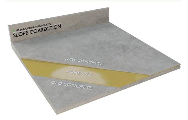
Slope correction, also known as resloping, is one of the repairs that can help preserve concrete structures. The need for slope correction can arise in various areas, such as balconies, elevator pits, and parking garage floors, where the existing slope may be insufficient or even inverted, leading to undesirable water flow patterns. For instance, improper slopes can cause water to accumulate towards the unit or garage walls, rather than draining away as intended.
